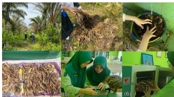
Gambar 1. Proses preparasi TKKS, meliputi: (1-2) Pengumpulan TKKS; (3) Pencucian TKKS; (4) Penjemuran TKKS; (5) Pengukuran massa TKKS; (6) Pengeringan TKKS.
