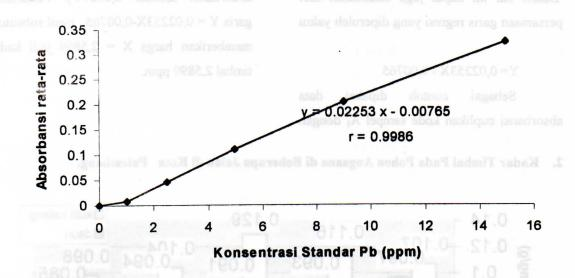
Gambar 1. Kurva kalibrasi larutan standar Timbal
