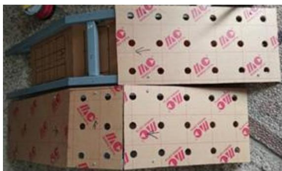
Gambar 1. Model Struktur Submerged Breakwater
